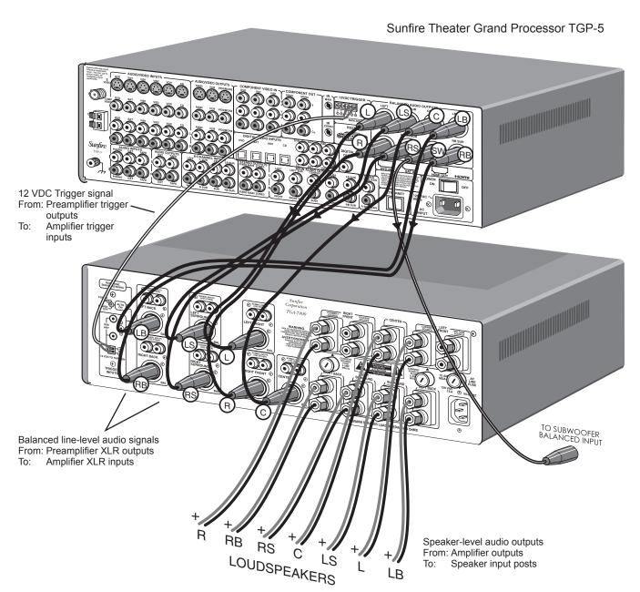
The 12 VDC trigger connection shown can be used to turn the amplifier on when the preamplifier turns on. Alternatively, you could use the amplifier's AUTO-ON switch. The amplifier will then automatically turn on when a preamp audio signal is received.
